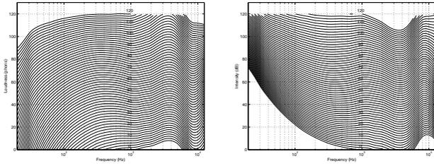
Figure 2: Top: Equal-SPL curves. Bottom: Equal-LL curves. From Eq. (13).
