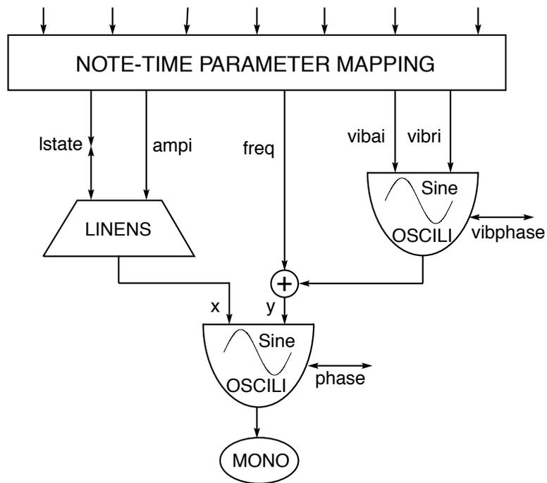
VibTone Instrument Flow Diagram
