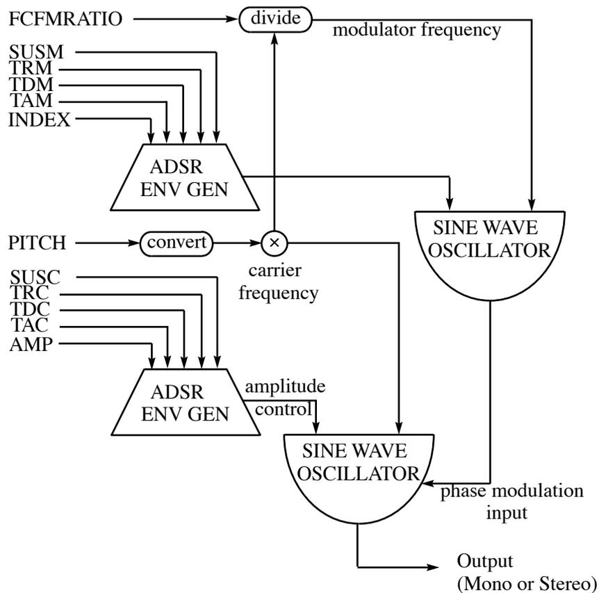
In the actual implementation of this flow diagram, for efficiency, the two sine wave oscillators are combined into a single phase modulation unit generator.
