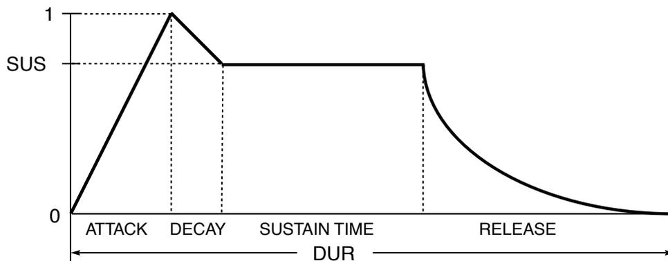
The four parameters for the ADSR are ATTACK, DECAY, SUS, and RELEASE. ATTACK, DECAY, and RELEASE are given in seconds, and their sum should always be less than the duration of the sound, DUR. SUS is the sustain level relative to the peak level (always 1.0) of the envelope. Therefore, SUS should always be in the range 0 to 1.0. The *sustain time* can be automatically calculated from the other times given using
